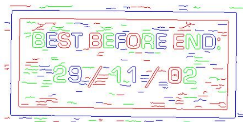
Figure 3.24: Segmentation of initial components with a too low contrast.
