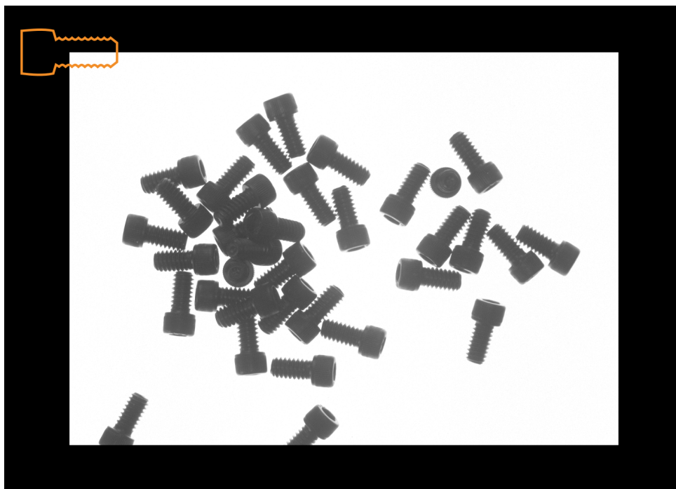
Figure 2.9: The model (orange) created from XLD contours contains negative coordinates.
